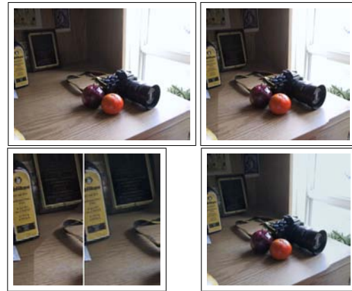
Figure 10: Seam Carving in the gradient domain. The original image (top left) is retargeted using standard technique (top right) and in the gradient domain (bottom right). Zoom in comparison is shown on bottom left.
